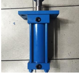
Gambar 3. 13 Silinder Hidrolik (Sumber: https://shorturl.at/k9Wmq )
