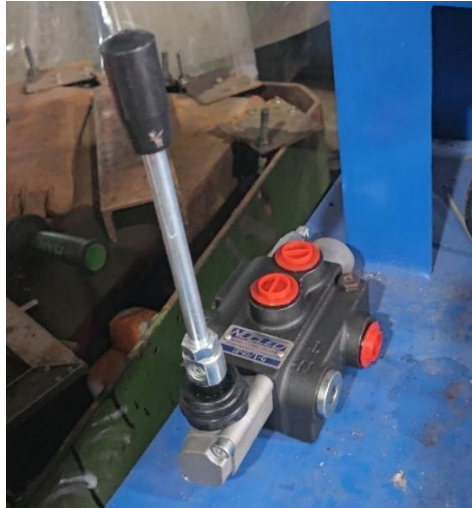
Gambar 3. 15 Directional control valve
