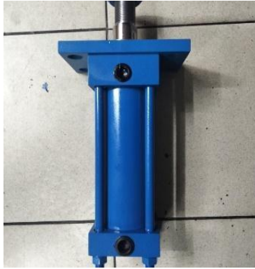
Gambar 3. 13 Silinder hidrolik (Sumber: https://shorturl.at/k9Wmq )
