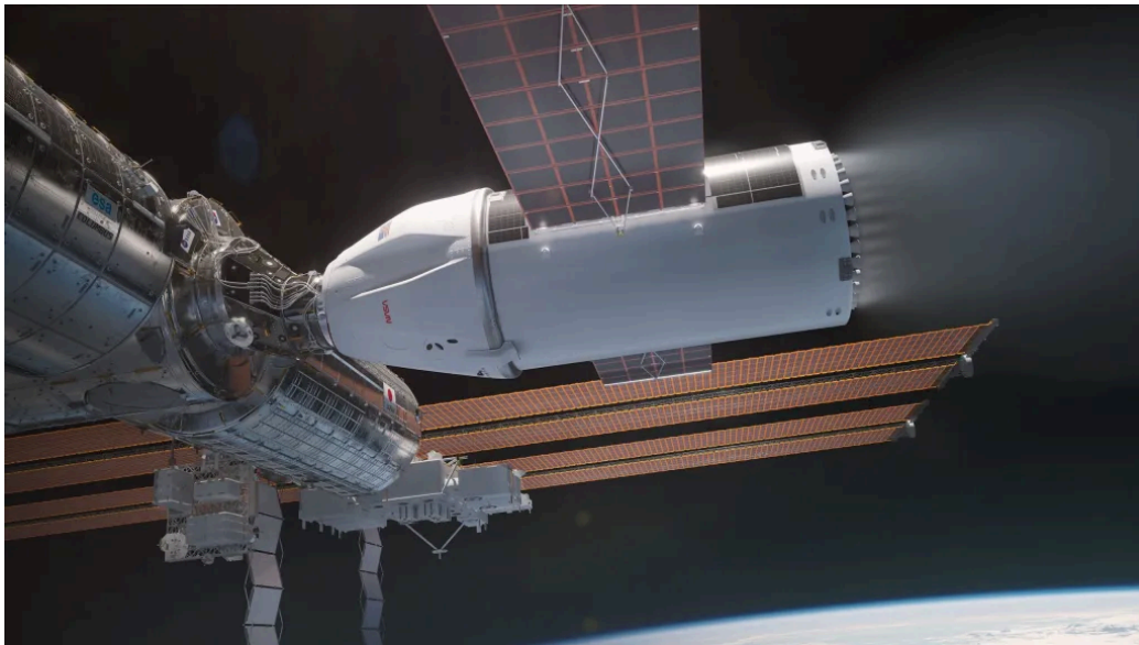
Gambar 2. 15 SpaceX's design of the U.S. Deorbit Vehicle is based on its Dragon spacecraft with an enhanced trunk section.
