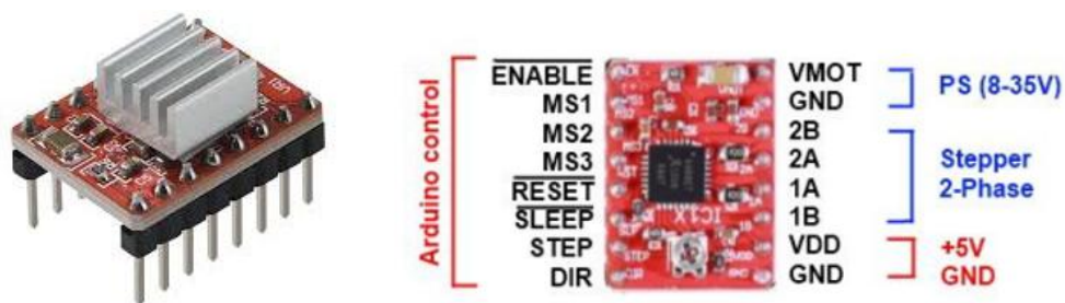
Gambar 2.7. Driver motor stepper A4988 dan pin I/O
