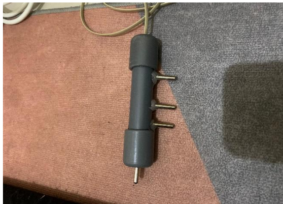
Gambar 2.10 Sensor Water Level
