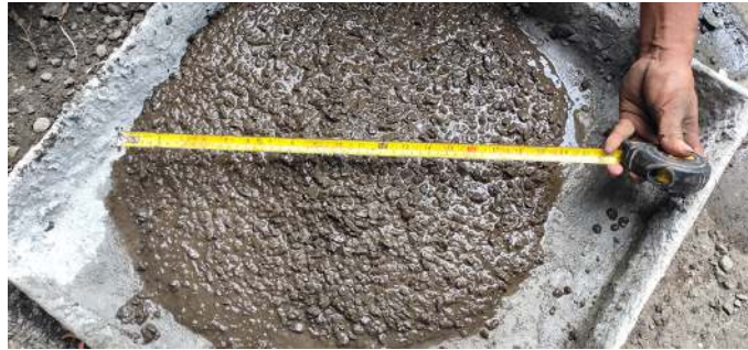
Gambar 3.8. Slump flow time beton geopolimer
