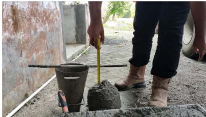
Gambar 3.9. Proses uji slump test beton konvensional
