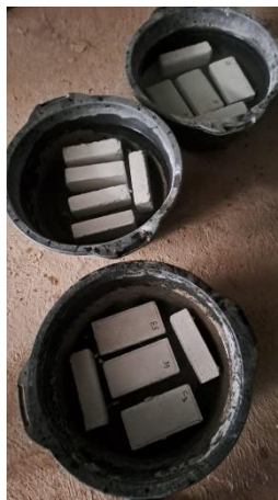
Gambar 3.52 Merendam Paving Block
