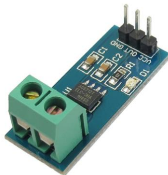
Gambar 2. 11 Sensor Arus ACS712
