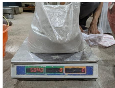
Gambar 3. 23 Penimbangan Semen Campuran Paving block
