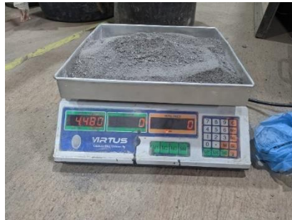
Gambar 3. 22 Penimbangan Pasir Campuran Paving block
