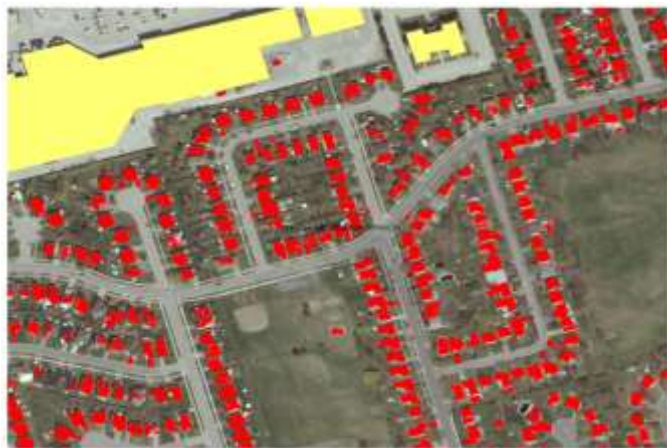
Gambar 2.8 Hasil ekstraksi lahan atap berbasis AFE ( Automated Feature Extraction )
