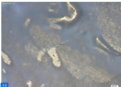
12 Fig. 9. Shows the results of the photomicrograph PVA-Collagen 1% image + Chitosan 10 drops
