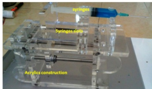
Fig. 3. Syringe electrospinning pump.
