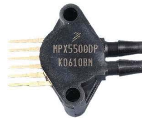
Fig. 7. Selected pressure sensor MPX5500DP
