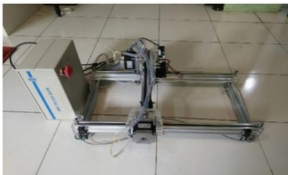
Gambar 4. Prototipe mesin CNC laser engraving .
